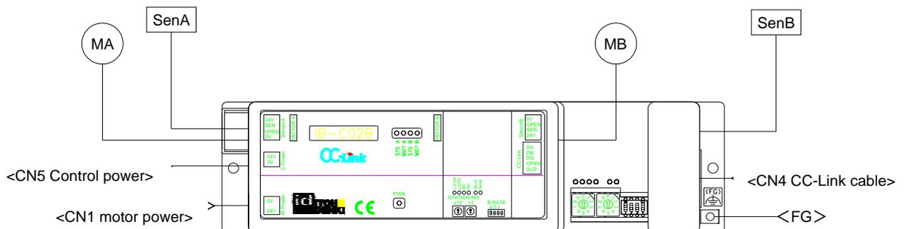
① Wire 24VDC and 0V to the motor power connector<CN1(2 poles)>
