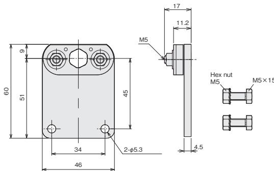
\*Attach to the power cable side.
