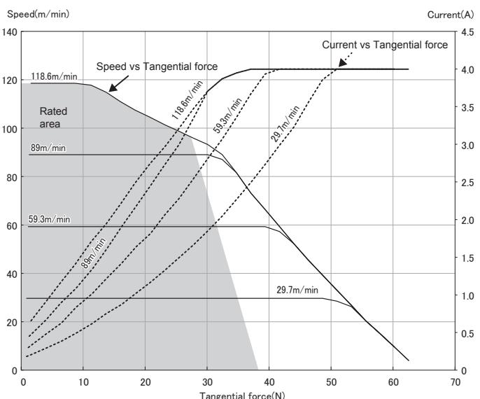
\* The values in the characteristics list are when an ambient temperature is 25 degree C, and only for your reference and not the warranted values. The values represent the characteristics of a single standard motor roller(no linked operation) without including other specifications, and the values may change when including other specifications or with linked operation.
