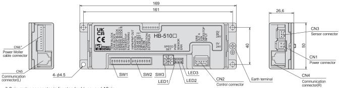
\* 9pin motor connector is for standard type, and 10pin motor connector is for brake function.
