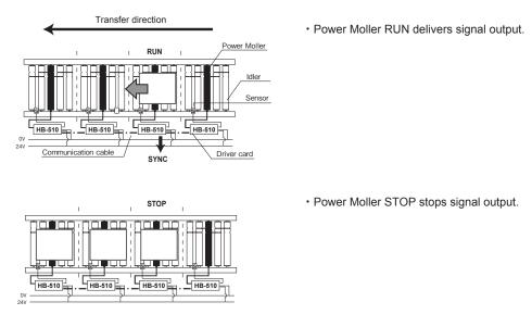
In addition, emergency stop function and sensor signal output function are also included.
