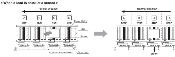
• [C] stops and generates error by the stuck load.
