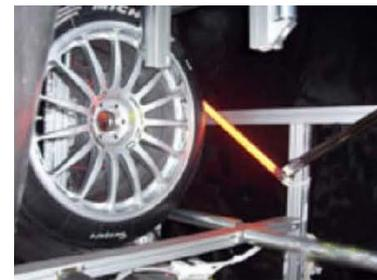
Heated tyres were subjected to scrutiny by heat cameras, showing that an equal distribution of heat was given and also that the generated heat remained in the tyre longer than if blankets had been used. The time taken to heat a tyre to 85°C and the hub to 60+°C took the Franc system less than 10 minutes to achieve - in comparison to 2 hours by blankets.
