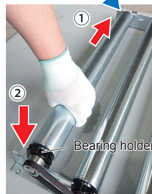
To stagger easily, tilt the idler slightly and mount
